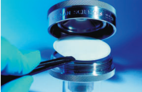
Composite membrane with selective nanoparticles for water purification
